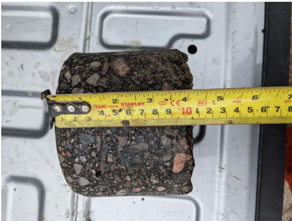
CH-1 Core, 100 mm total thickness, 2024
