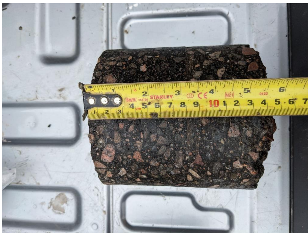
CH-10 Core, 140 mm total thickness, 2024
