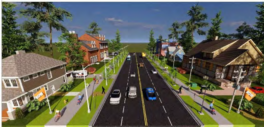
MAJOR URBAN ARTERIAL ROAD (36 m ROW) TYPICAL CROSS SECTION
